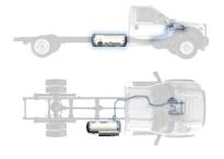
**Centre chassis tanks** are typically found on school buses and beverage trucks. They feature two long tanks in the centre of the chassis, with tank size options ranging from 75 to 150 litres (Type A – Short Bus) and 250 to 350 litres (Type C – Traditional School Bus).
